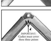
\*Step 3: Align duct, insert screw, and tighten
