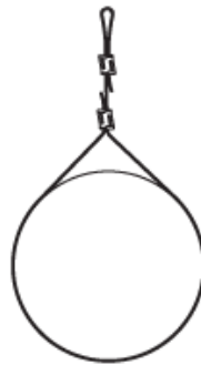
FIGURE 5—HANGING METHOD – STANDARD LOOP CONFIGURATION
